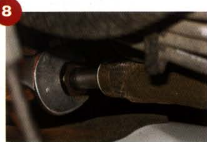
Next, the EGR tube was removed from the rear of the driver's side manifold.
