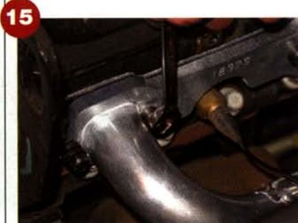
New hardware is used throughout to attach the header to the head.
