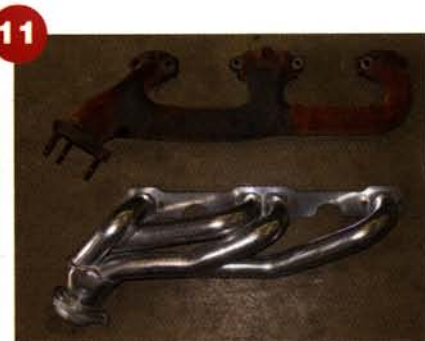
A side-by-side comparison makes the superior flowing capabilities of the JBA unit pretty obvious.
