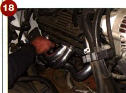
The manifold was removed and the header quickly replaced it.
